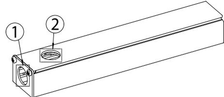
Subsequently, depending on the hole used, make a hole to pass the cable through the end cap or track.
