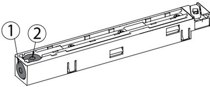
Apply force to removable section 1 or 2 and feed the power cable through the resulting hole.
