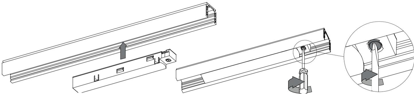
Lastly, insert the power end feed into the track (Pic. 8) and secure it by means of device B fitted on it, by turning until it stops (using an appropriate screwdriver).
