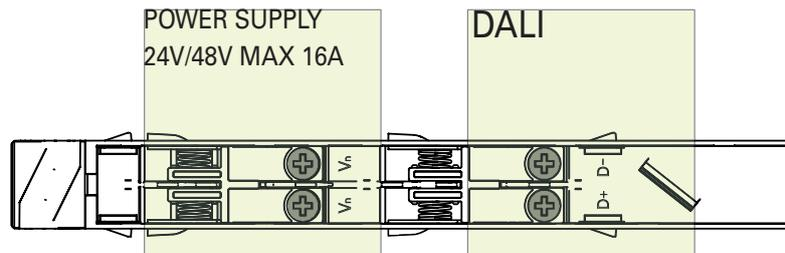
Remove the cable sheaths and strip the cables, then wire the contacts of the end power feed taking care to respect the markings on it ( $V_n/+/-$ ). After completing the operations, use the screw-mount cable clamp located on the power end feed, put the cover back on and tighten the 3 screws A1-A2-A3.
