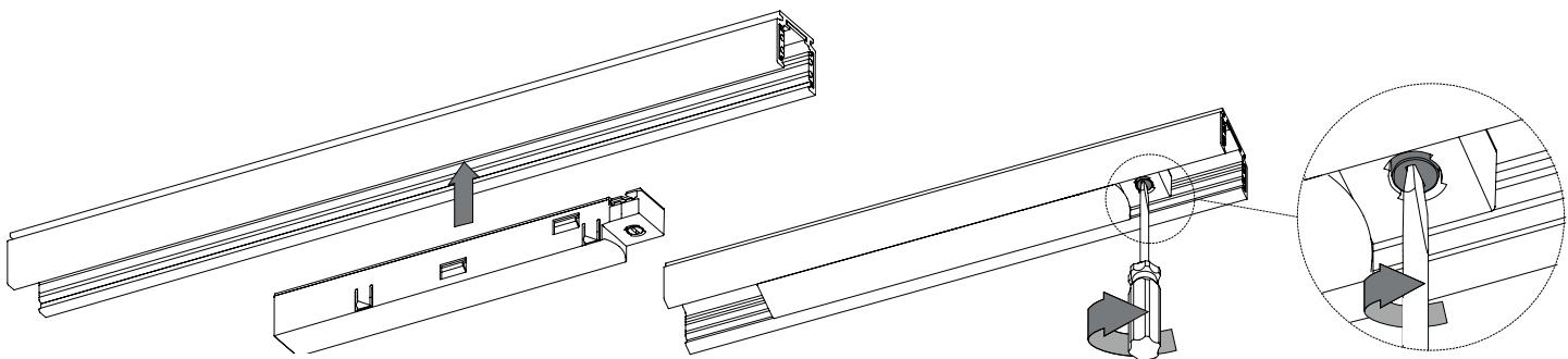
Lastly, insert the power end feed into the track (Pic. 8) and secure it by means of device B fitted on it, by turning until it stops (using an appropriate screwdriver).
